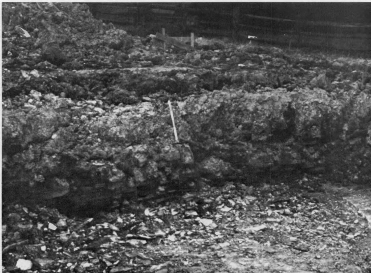
FIGURE 15.—Lacustrine clay approximately 3 feet thick on Berea Sandstone (bedrock unit II) overlain by modern soil in clay at construction site on Escarpment at Independence. Photo taken in April 1974.
